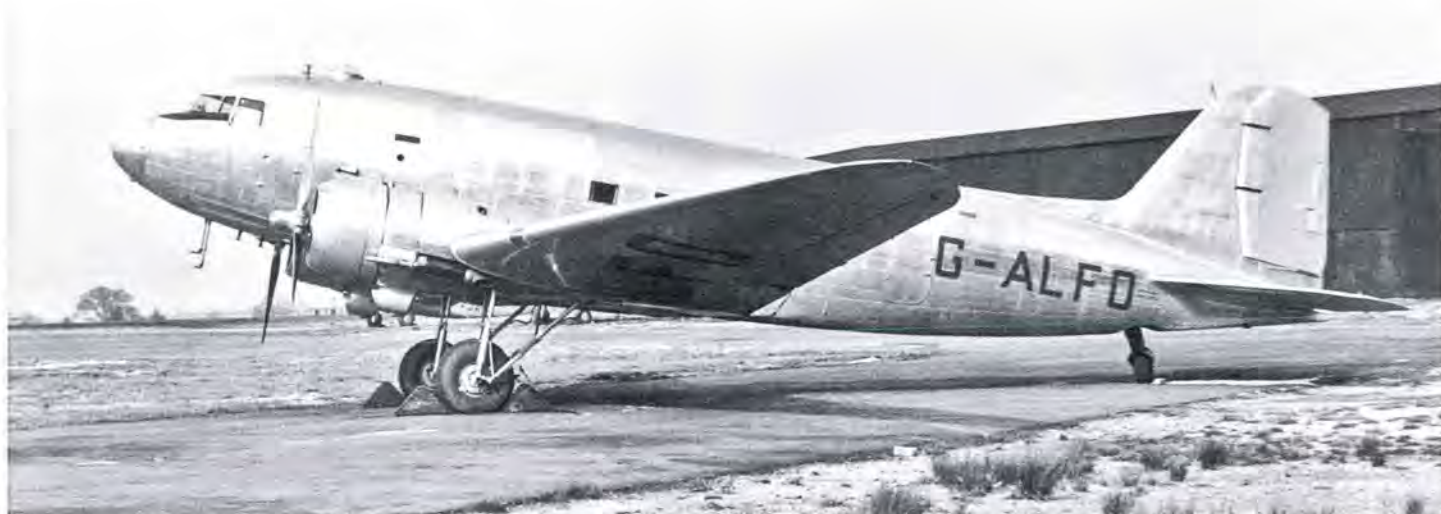
DC-3 VH-BHC after British certification as G-ALFO. The metal reskinning of the forward fuselage is clear in this view, but the purpose remains obscure. (A.J.Jackson)
