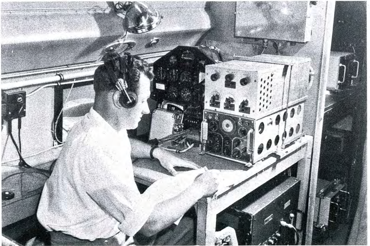
Magnetometer operator's console in the cabin of Bureau of Mineral Resources DC-3 VH-BUR (the former VH-BHE) soon after it commenced survey work in 1952. The operator is BMR specialist John Newman, who had adapted a wartime aerial anti-submarine Magnetic Anomaly Detection (MAD) system. (Ted McCarthy via Doug Morrison .)
