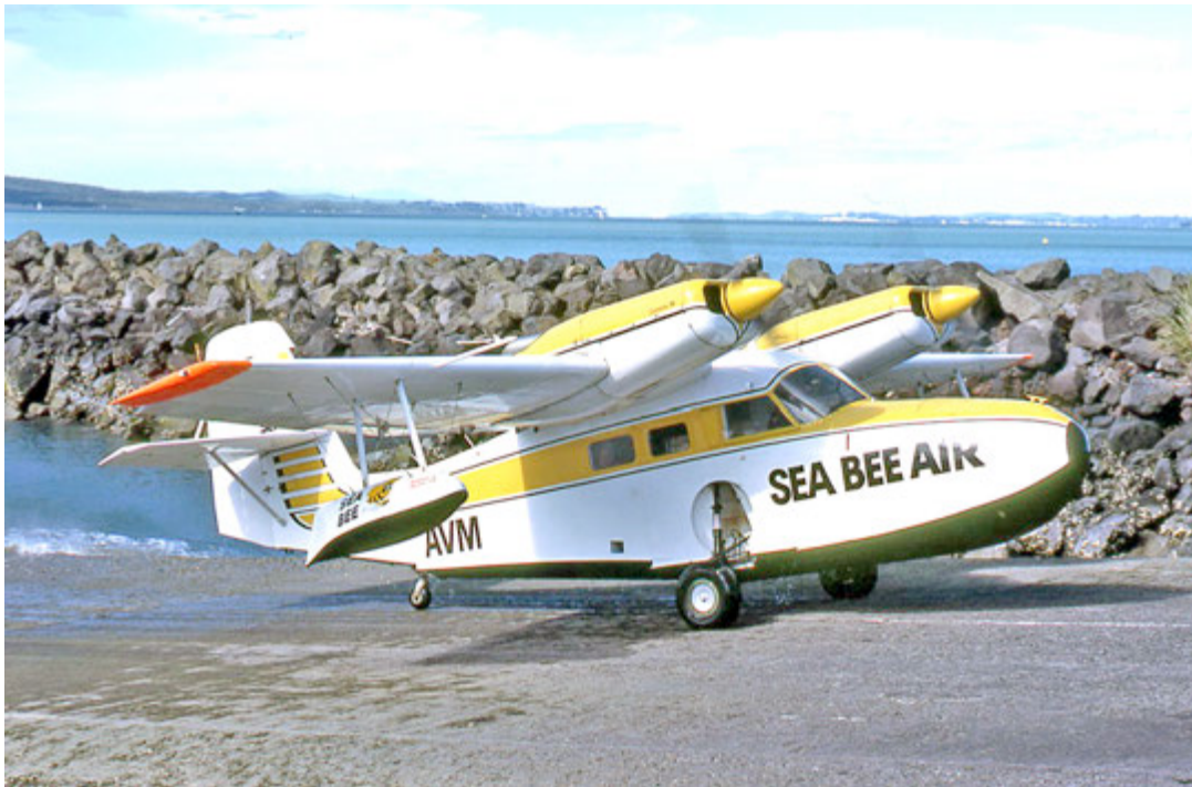
ZK-AVM (c/n 1466) at Auckland Harbour NZ in October 1977. This was rebuilt in NZ to the McKinnon Enterprises Super Widgeon conversion with 260hp Continental IO-470 flat-six engines. Photo by Geoff Goodall
