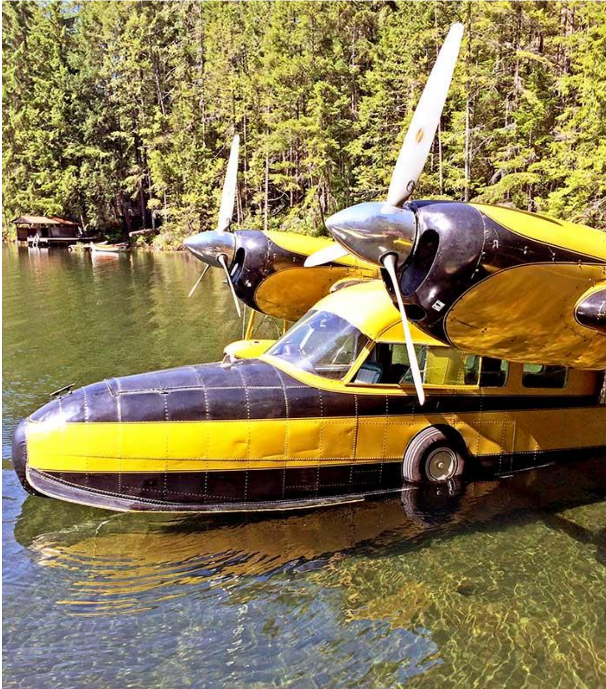
CF-ODR seen at Boundary Bay BC in 2015 was c/n 28 of 41 production SCAN-30s, French licence-built Widgeons. Many migrated to North America where they they were rebuilt with more powerful engines and a range of modifications to enhance performance, just like the Grumman Widgeons. Photo courtesy owner Mark Williston
