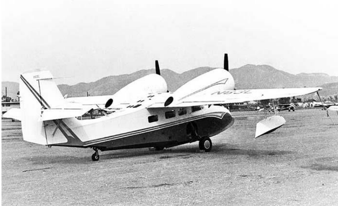
This view of N63L at Whiteman Air Park CA in January 1961 highlights the size of the Lycoming 680E radial installation of the Gannet Super Widgeon modification. Photo by Barney B. Deatrick
