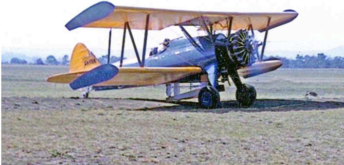
Crop-Care Pty Ltd National NA-75 VH-FBA giving demonstration flights at Armidale NSW in October 1957. The large US designed spreader can be seen under the belly. Photo: John Patterson collection
